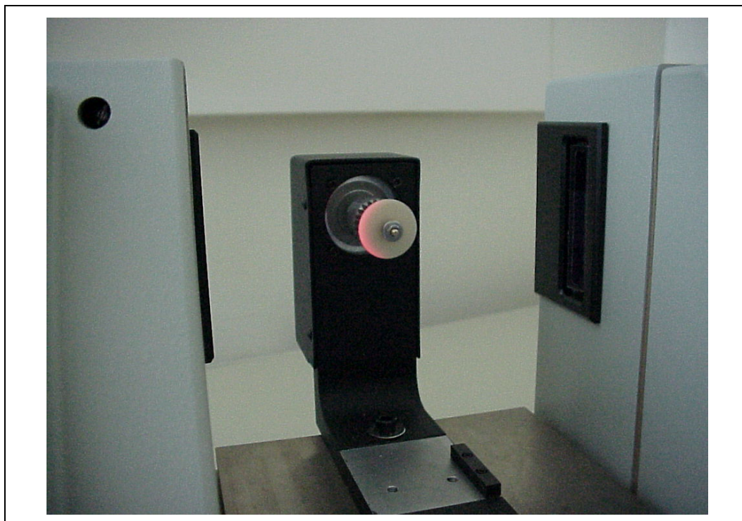
Figure 4 An Expansion Disc being measured with a Laser Micrometer
